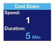
4. Press the UP or DOWN button to select the SPEED # for COOL DOWN; then press the MENU button to select DURATION in minutes; then press the RETURN button twice to get out of SWIM WORKOUT.
