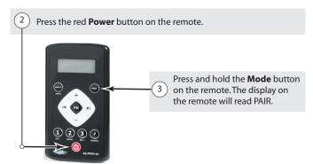
While still holding the **Mode** button, press and hold the **Power** button inside the docking station for <u>five seconds</u>.
