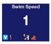
5. Press the SWIM WORKOUT button to turn ON the pump – the red SWIM icon on the LCD screen turns ON. The WORKOUT feature will activate to cycle each of the SPEED setting and specific DURATION setting for WORKOUT. If you need to increase or decrease the pump speed manually; then press the UP or DOWN button to your desired SPEED # in each cycle.
